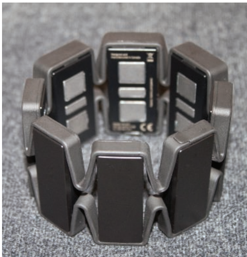
The Myo armband, which can currently be fashioned in either black or white, expands to fit any arm larger than a typical 12 year old.
